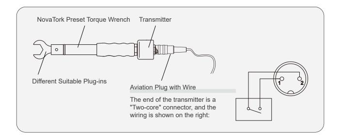
Note: The wired transmitter can be used with most NovaTork preset torque wrench of PC / PCH series. If you need it, please consult the supplier.
